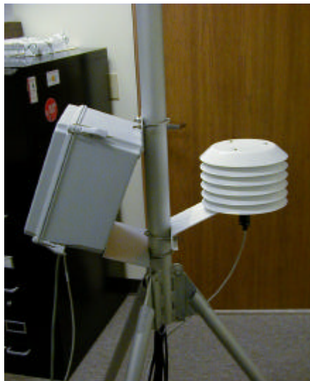
Figure 2.3 Control Unit and Temperature Sensor Assembly
